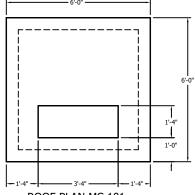
**ROOF PLAN MC-101** (75-500 KVA TRANSFORMER COVER)
