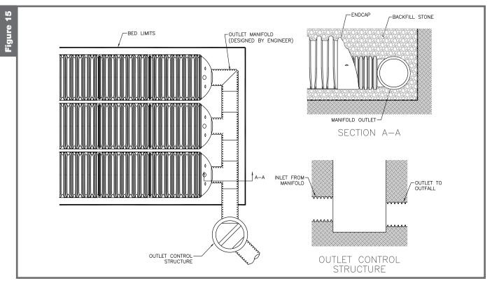
Note: Engineer is to specify the elevations of the piping, stone, and chambers.
