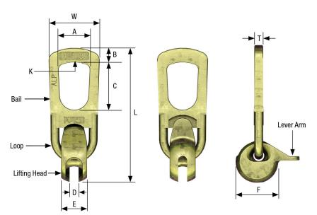
Designed as an attachment link for lifting and transport of precast concrete units in combination with the ALP® Lifting Pin Anchor System. The Lifting Eye consists of a Lifting Head with a protruding lever arm and a high strength Bail. The Lifting Head has a "T" slot that engages the head of a Lifting Pin Anchor. The rotation capabilities allow the lifting eye to stay oriented in the direction of loading without binding up.
